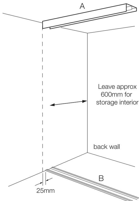
**Top Track** - Position the Track into the top of the opening. Mark where holes need to be drilled in the track (we recommend a fixing at each end and centre then at regular intervals in between). Drill and plug the header/ceiling in line with the holes drilled in the track and fix the top track using the long screws provided (see back page for suggestions).
