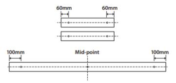
Drill pilot holes through the shelf bearers from each end at the distances shown, and one pilot hole at the mid-point of the back shelf bearer, after it has been cut to length.
