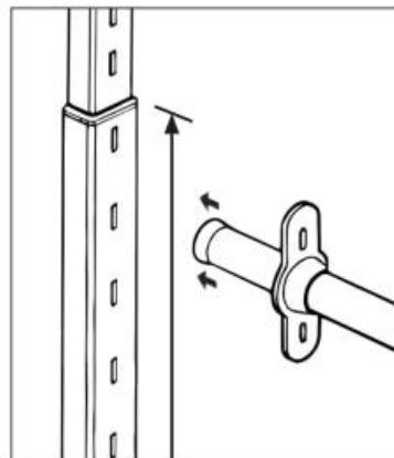
UK: For maximum weight bearing capacity, the hanger bar should be fixed between the non-extendable parts of the supporting stanchions.
